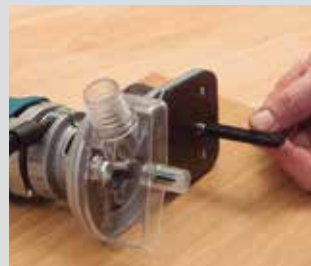
Corner trimming device easy to prepare and to use. When not in use it can be hidden into the base.
