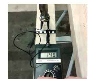
Fig. 3: Wood moisture measurement after leak-tightness test
